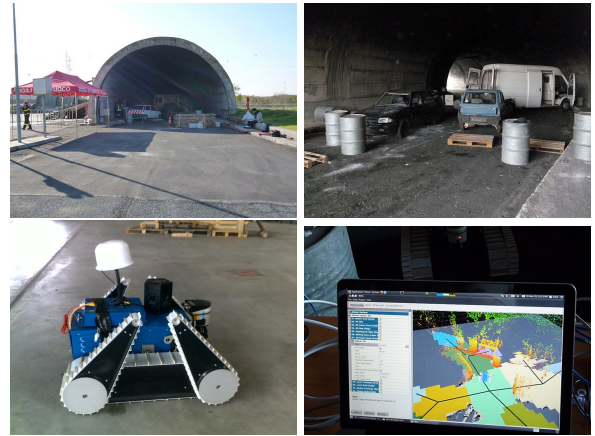
Fig. 12 Pictures of the tunnel accident environment. Upper row: Left: entrance of the tunnel, right: in the middle of the environment with barrels, pallets, and damaged vehicles. Lower row: Left: the robot used for the tests, right: A live screen during one test.
