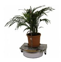
**Fig. 1.** Prototype of the cyborg, the final version will feature a casing hiding the electronics.
