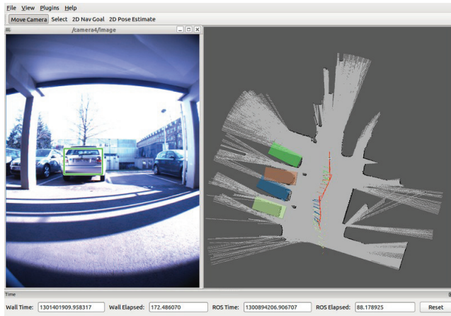
Figure 2: Example of car detection in one of the LB3 cameras and car models placed in 3D map.
